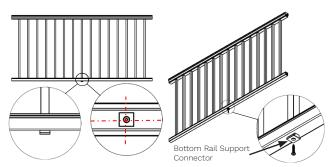
Note: For shorter sections, Remove an additional 5/16"(8mm) on both ends (5/8"(16mm) overall) for the bracket to fit between the rail and post. Trim the top and bottom rails to length.
