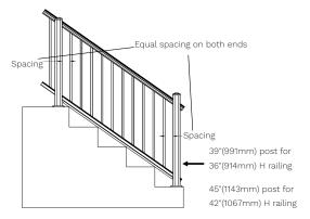
Note: During installation, please don't tilt the railing to the maximum angle repeatedly as this will scratch the powder coating on the pickets.
